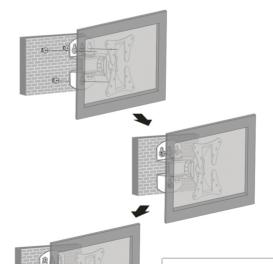
Step 4. Gently hang the screen on the screws. Before releasing the suspended screen, make sure that bracket holds firmly. Tighten the screws with a screwdriver.
