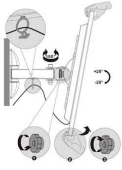
Step 6 In order to change tilt angle use knob on the bracket arm. Tighten it back after setting desirable TV position.
